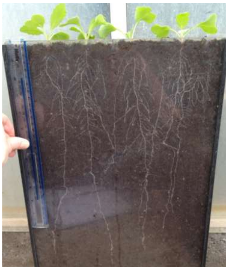
Figure 2 Radish plants growing in a rhizotron allowing measurement of roots
