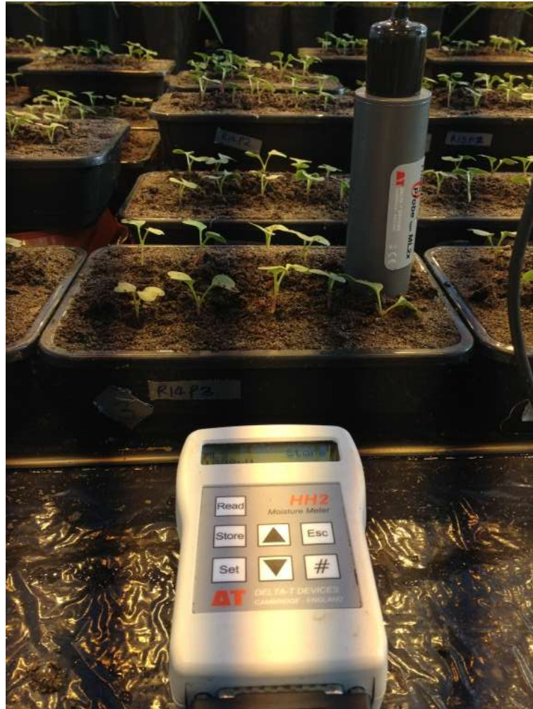
Figure 7 Measuring the volumetric water content of the compost in a plant pot using a Theta Probe
